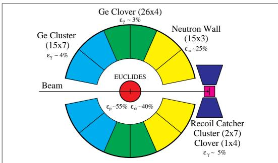
Figure 7.6: Schematic drawing of the set-up for isomer tagging at IReS, Strasbourg, during the Neutron Wall campaign in 2001.
