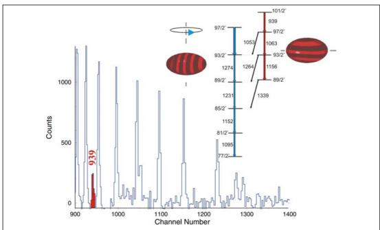
**Figure 5.2:** EUROBALL spectrum and level scheme for the top of the (+, +1/2) band in <sup>159</sup>Er. The 939 keV gamma ray is the transition depopulating the fully aligned band termination state at  $101/2^+$ .
